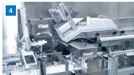
The wallets are transferred in stacks of seven to the Uhlmann C 200 cartoner.
