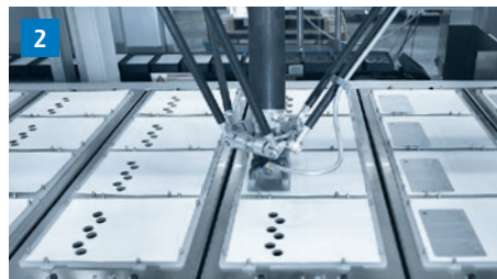
The KS-PL wallet machine from KOCH seals the blisters with front and cover cards to create childproof, yet senior-friendly wallets.
