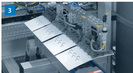
A completely newly developed folding system allows many axis movements and can handle the enormous variety of blister formats.
