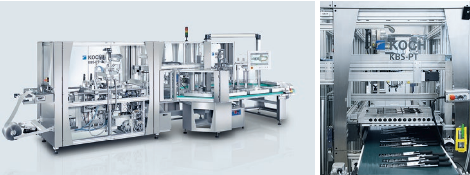
The KBS-PT Blister Machine is ideally designed for quick format changes, high packaging capacity and top flexibility when processing different formats and materials.
